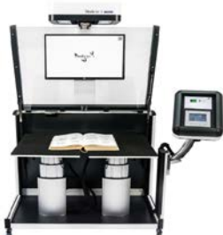
Figure 4: A planetary scanner for use with ancient manuscripts
